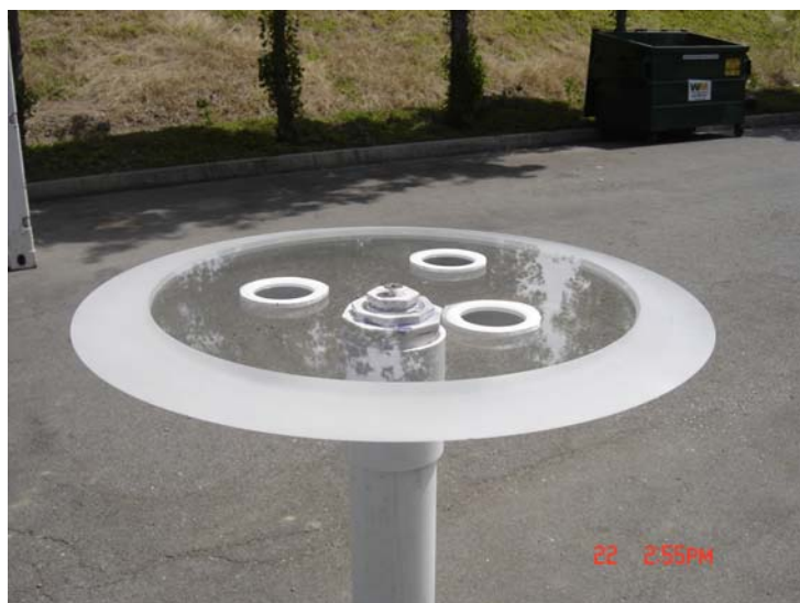
Figure 4-3. View from above the Aerodynamic Deposition Plate Showing Three Positions Available for the Sample Cartridges
