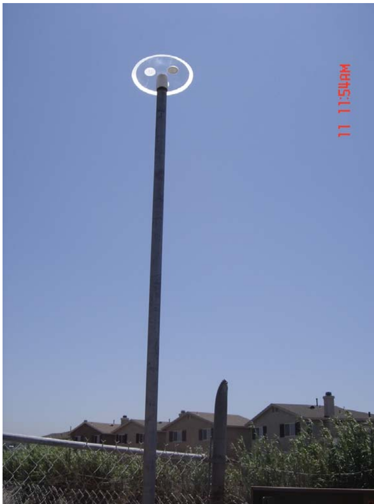
Figure 4-4. Aerodynamic Deposition Plate Mounted on the Rain Gauge Pole at Site DPR(2)
