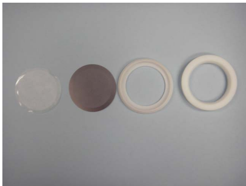
Figure 4-8. Teflon Sample Disk (left) and Passive Sampler Cassette Parts, Backing Screen (second from left), Base (second from right), and Top (right)
