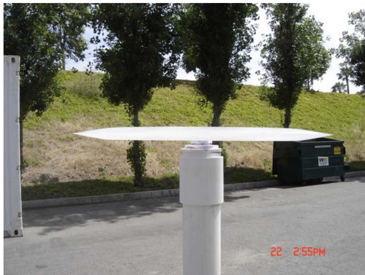
Figure 4-2. Cross Sectional View of the Aerodynamic Deposition Plate – Leading Edge is at a 10° Angle
