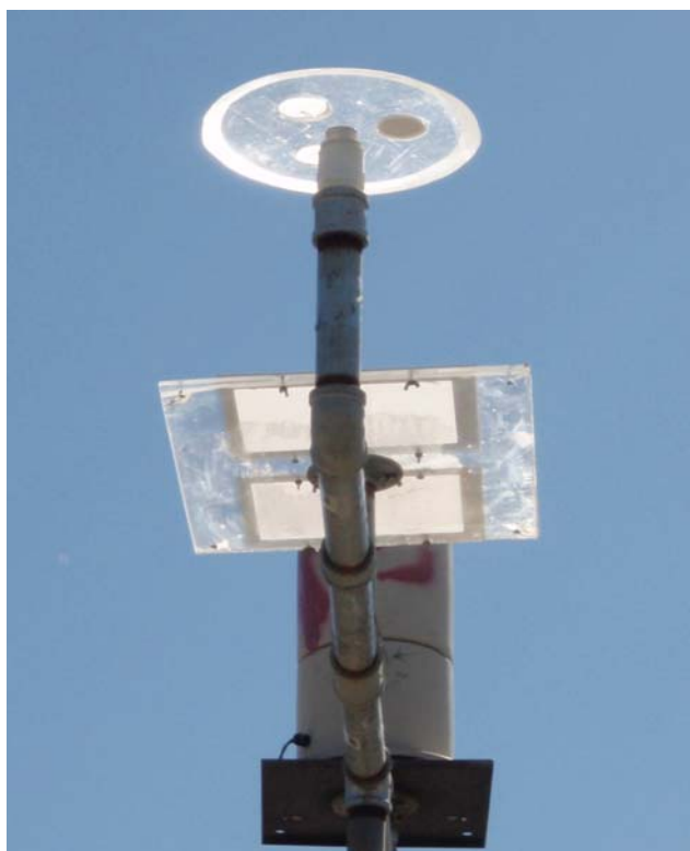
Figure 4-11. Particle Solubility Apparatus Mounted with a Surrogate Sample Disk Apparatus at Site SD8(1)
