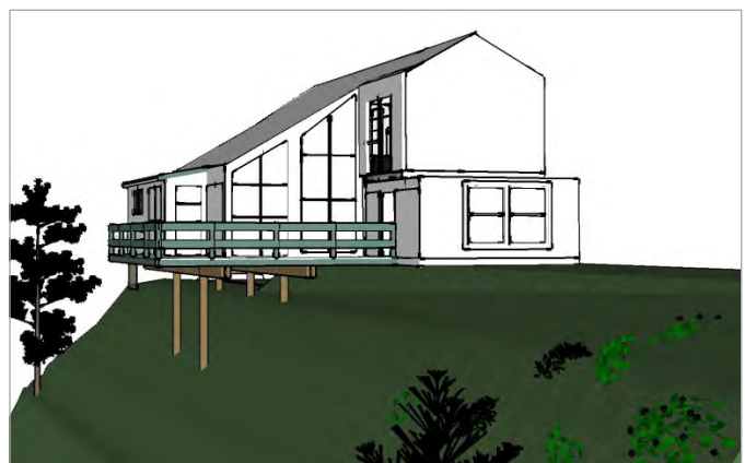
Illustration of policy UD-3.55(c): Minimize grading.
