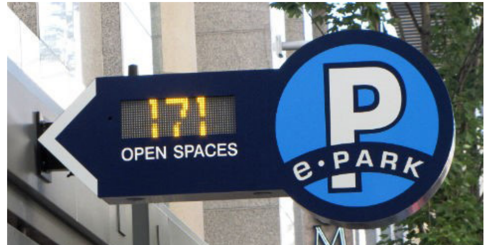
Real time parking information at this parking garage provides the number of spaces available and can be linked to a smart phone for efficient access to parking.
