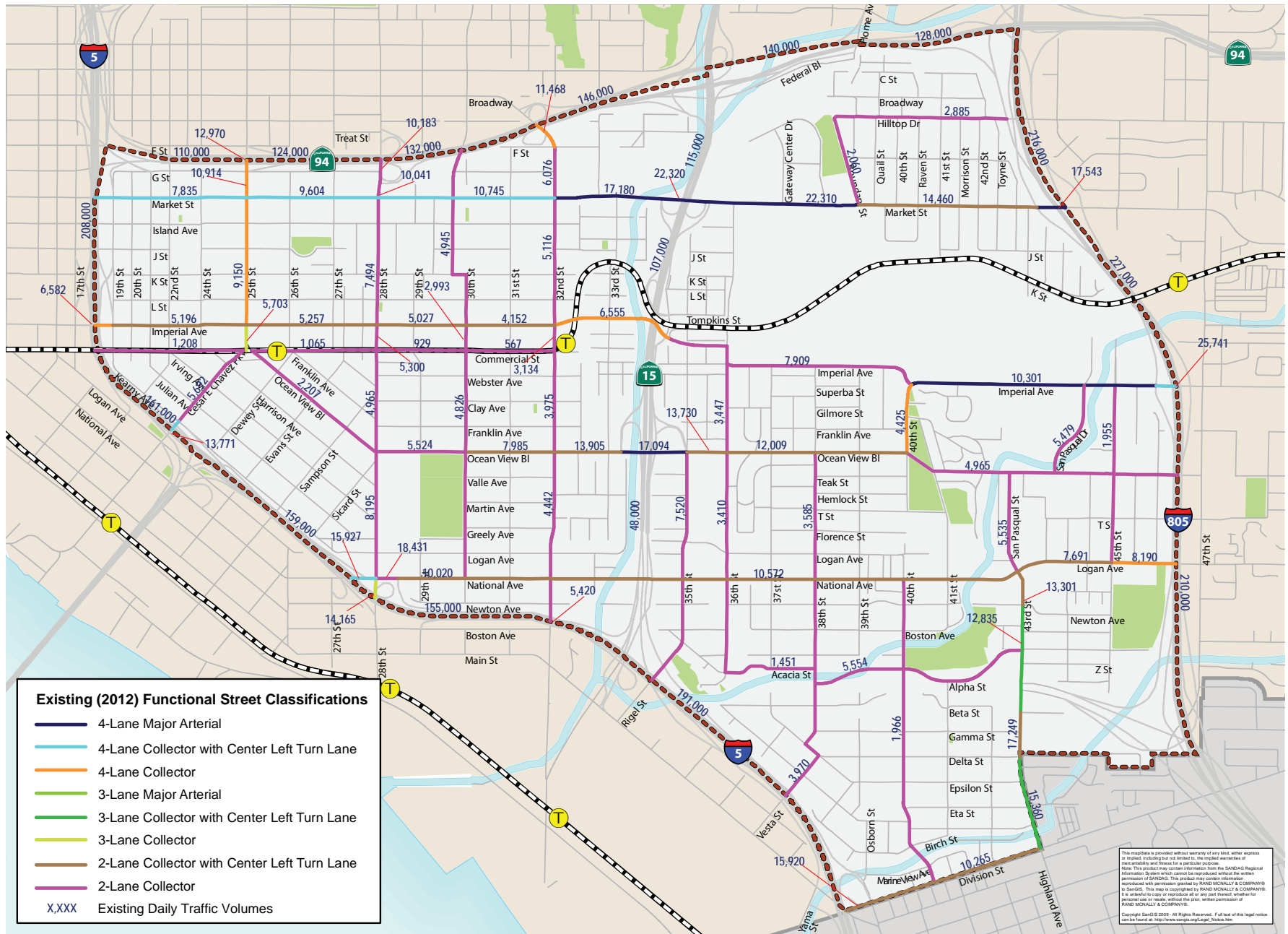
FIGURE 3-7: Existing (2012) Functional Street Classifications and Daily Traffic
